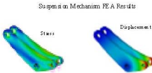
Figure10: Bellcrank FEA results
