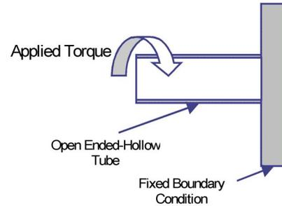
Figure 19: Torsion Tube
