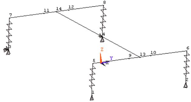
Figure 9: Vehicle Stick Model – Compliant Springs
