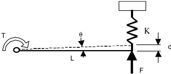
Figure 8: Linear to Torsion Spring
