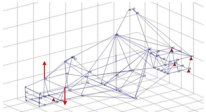
Figure 20: Frame Finite Element Model Loading Case
