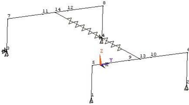
Figure 10: Vehicle Stick Model – Compliant Frame
