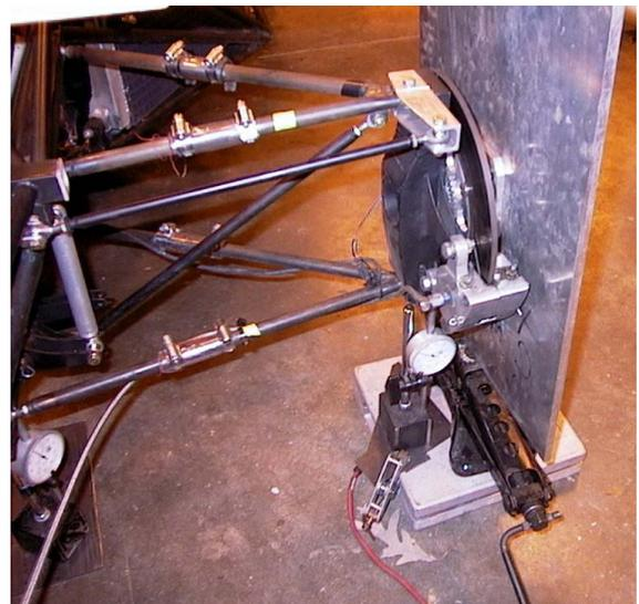
Figure 23: Testing Setup for Front Left Corner
