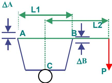
Figure 22: Front Suspension Bay Testing Loads
