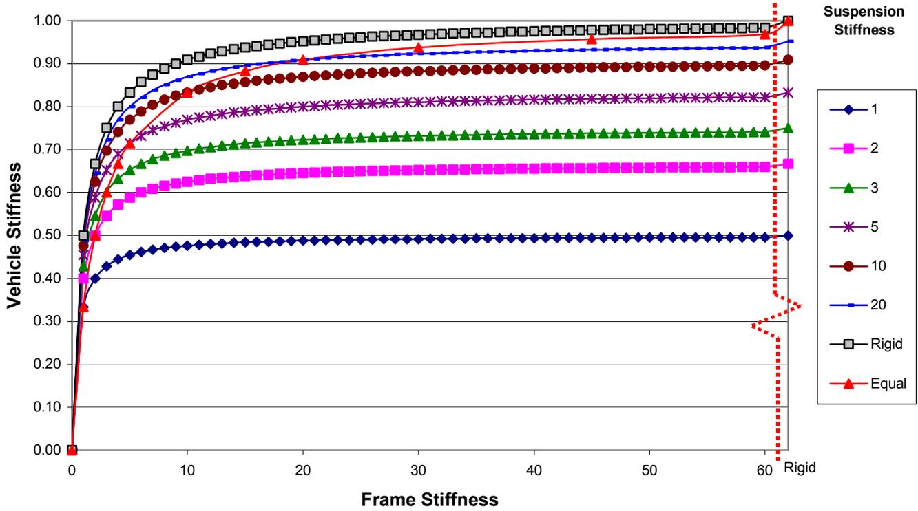
Figure 13: Normalized Chassis Stiffness for Varying Frame and Suspension Stiffness
