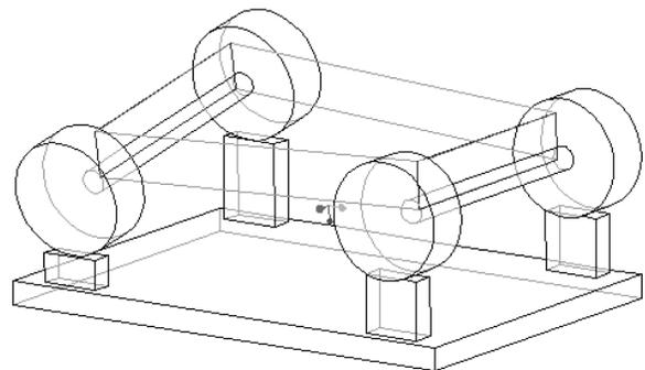
Figure 1: Longitudinal Torsion Deformation Mode
