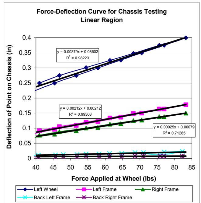
Figure 25: Twist Test Force-Deflection Curve Linear Region
