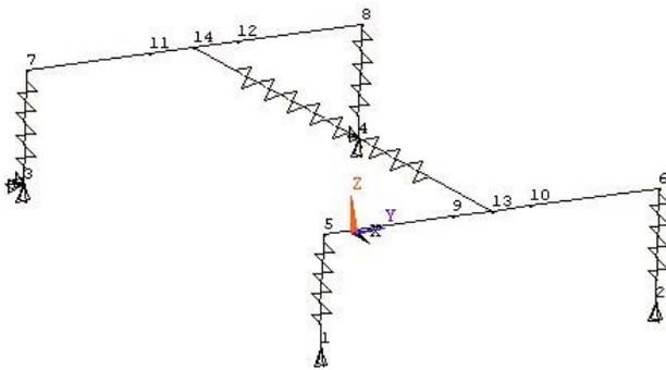
Figure 11: Vehicle Stick Model – Compliant Springs and Frame
