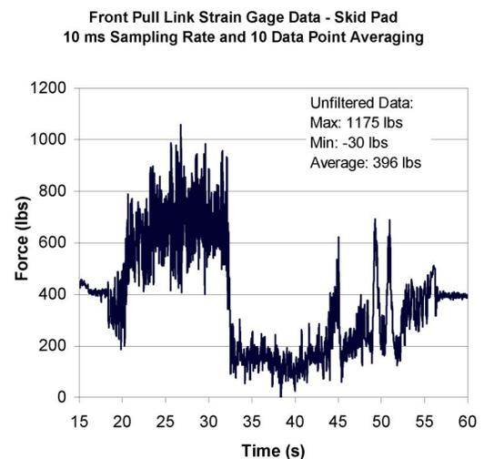
Figure 5: Strain Gauge Data
