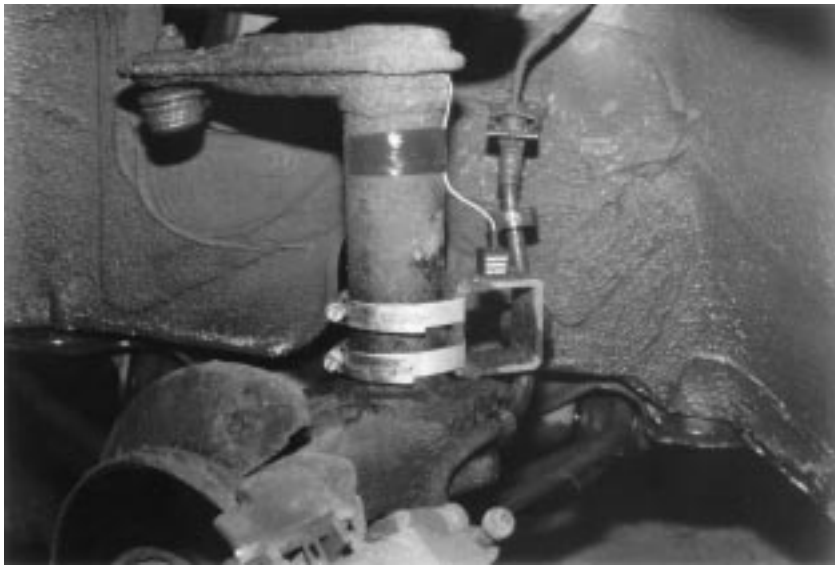
Fig. 4 Photograph of an accelerometer mounted on a suspension strut
