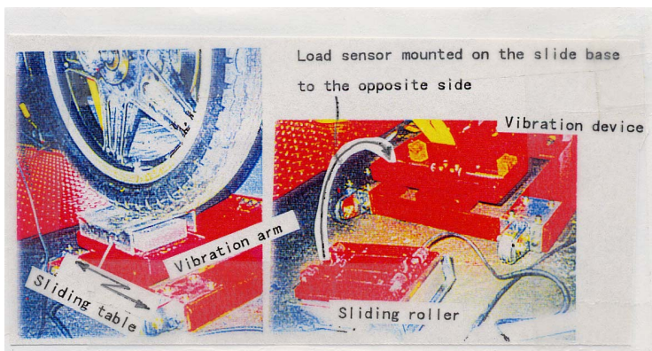
Figure 13 Sliding mechanism of before and after
