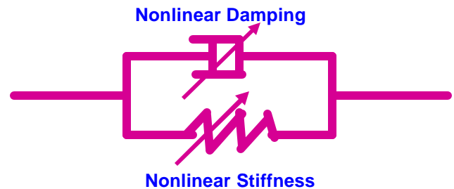
Figure 2: Nonlinear Element Formulation in MSC/NASTRAN
