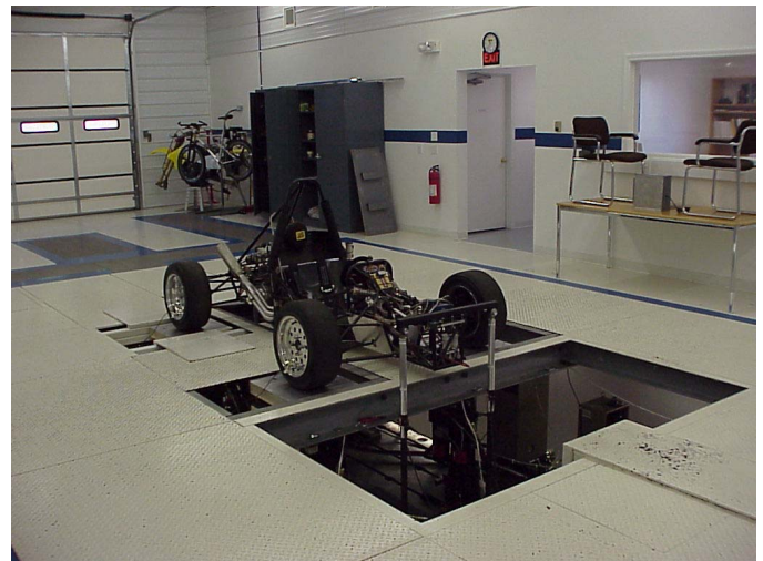
Figure 1. Clemson Formula SAE racecar setup on the seven-poster dynamic simulator.
