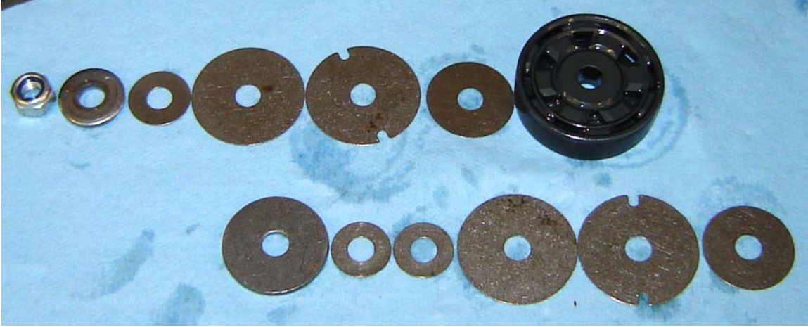
Figure 4. The upper set of plates is for the rebound side of the piston, while the lower set is for the compression side. Each shim performs a different function that influences the curve. The plates against the piston affect the preload on the whole stack, this will adjust the location of the knee of the curve. The plates with the slots are the bypass plates which determine the low speed forces. The large plate defines the overall magnitude of the curves. The last set of plates is for adjustment of the high speed region of the curve.
